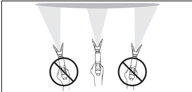
Keep the spray gun perpendicular to the surface, otherwise one end of the pattern will be thicker than the other.
