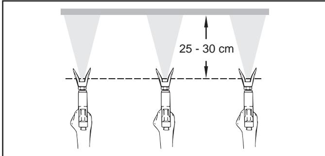
Keep the spray gun at right angles to the surface. This means moving your entire arm back and forth rather than just flexing your wrist.
