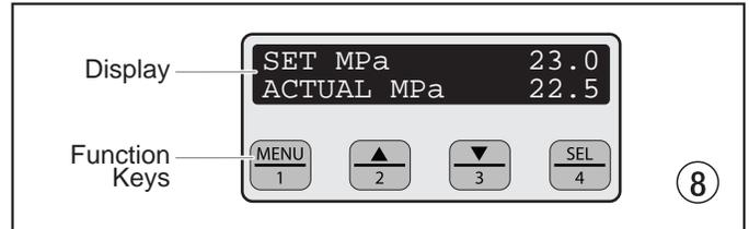
**i** The pressure control knob overrides the Digital Electronic Spray Control (DESC) settings. Anytime the pressure control knob is turned, the sprayer pressure will change accordingly.
